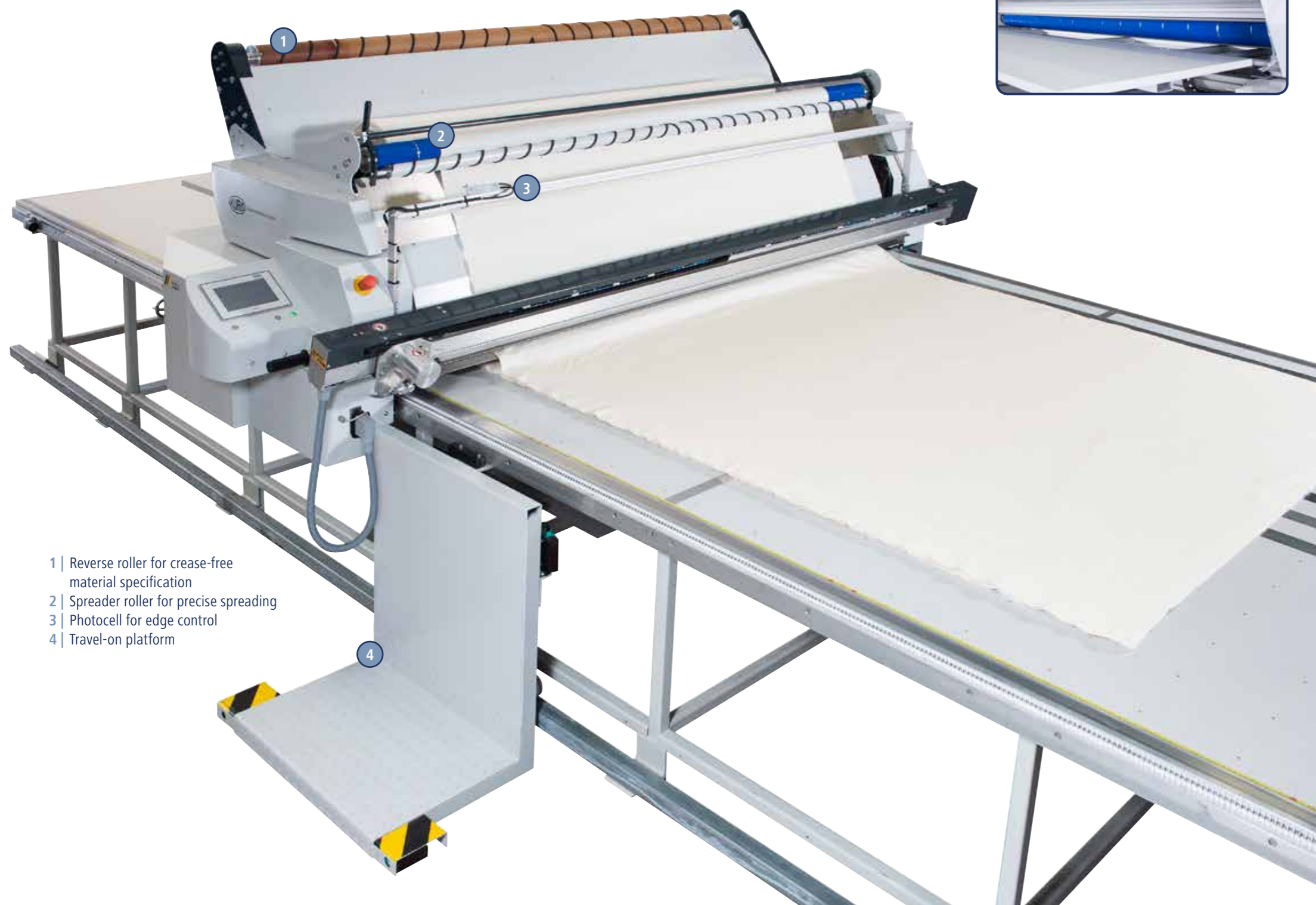
Touch panel with graphical interface for easy and clear operation.
